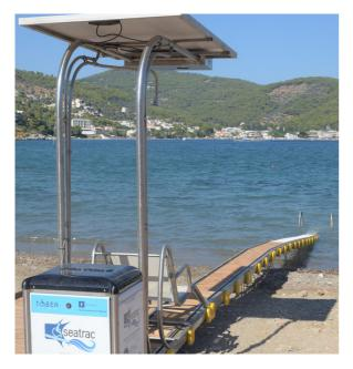
The system consists of the solar powered conveyance track that is totally controlled by the user. The system provides a fixed track chair that can be moved into and out of the water if someone chooses to take a swim or just get them to the water's edge. The system also provides a series of services -like signage options, a changing room and storage shed- that allow its users to enjoy a day at the beach.
