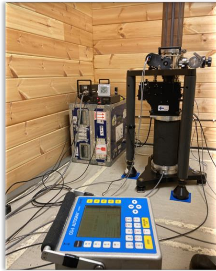
Figure 2: Two different gravimeters at the Kivetty station. On the back is an absolute gravimeter FG5X-221 (Micro-g LaCoste) and on the front is a CG-5 relative gravimeter (Scintrex).
