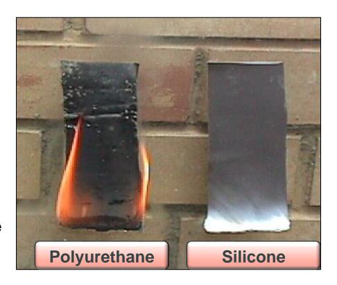
Silicones can NOT be categorized as non-flammable as they are not inorganic Silicones provide excellent fire retardant properties compared to other sealants
