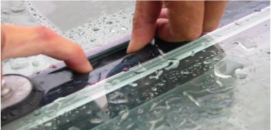
no or poor edge deletion of soft coating has cause adhesion failure of secondary sealant
