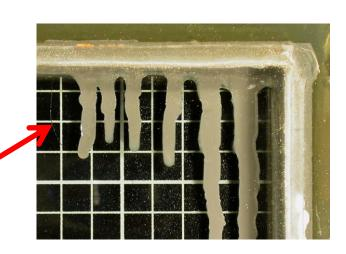
Delamination due to incompatibility: Highly diluted sealant has been used
