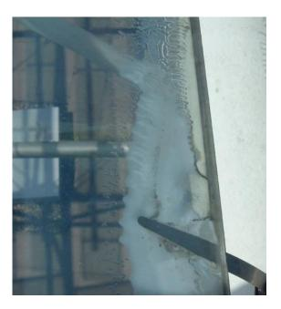
Plasticizer Migration Sealant to laminate & Laminate to sealant
