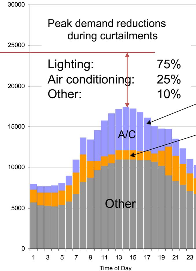
**30% Peak Savings Possible from Cooling Load Control and Daylight Dimming**
