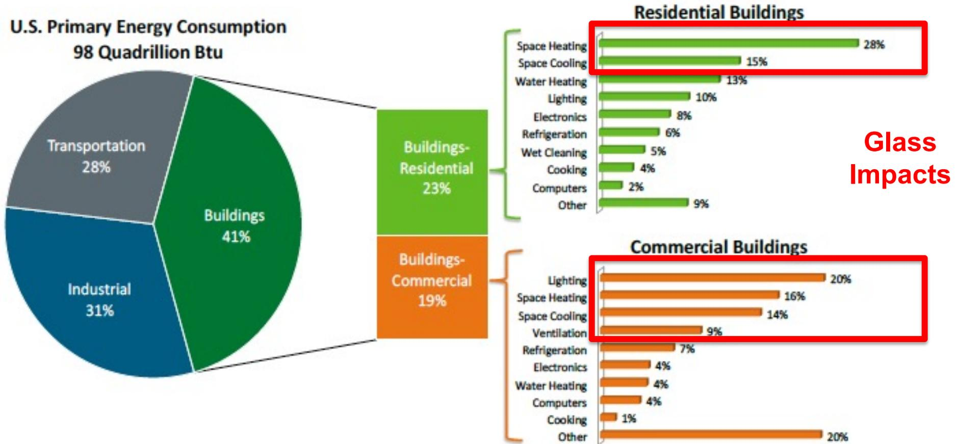
**Window “impact” on building loads ~ heating, cooling, lighting = ~40%
