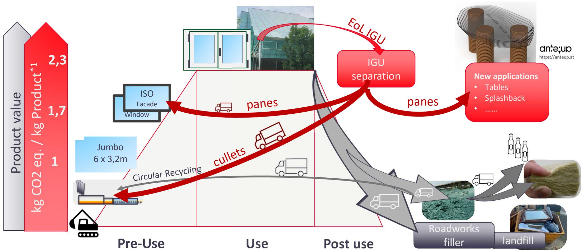
We develop the technology to establish circularity for IGU / construction glass
