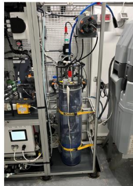
IFCB, automated plankton sampling every ~25 minutes AI-assisted analysis
