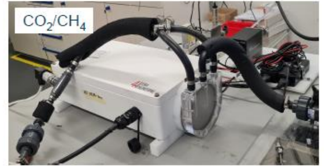
HydroC® CO2/CH4 Combi FT connected to the calibration unit
