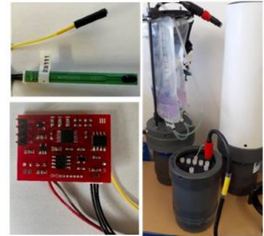
Lab-on-chip pH sensor combined with an electrochemical ISFET-type pH sensor enabling fast, high-accuracy measurements on fast-moving platforms such as gliders.
