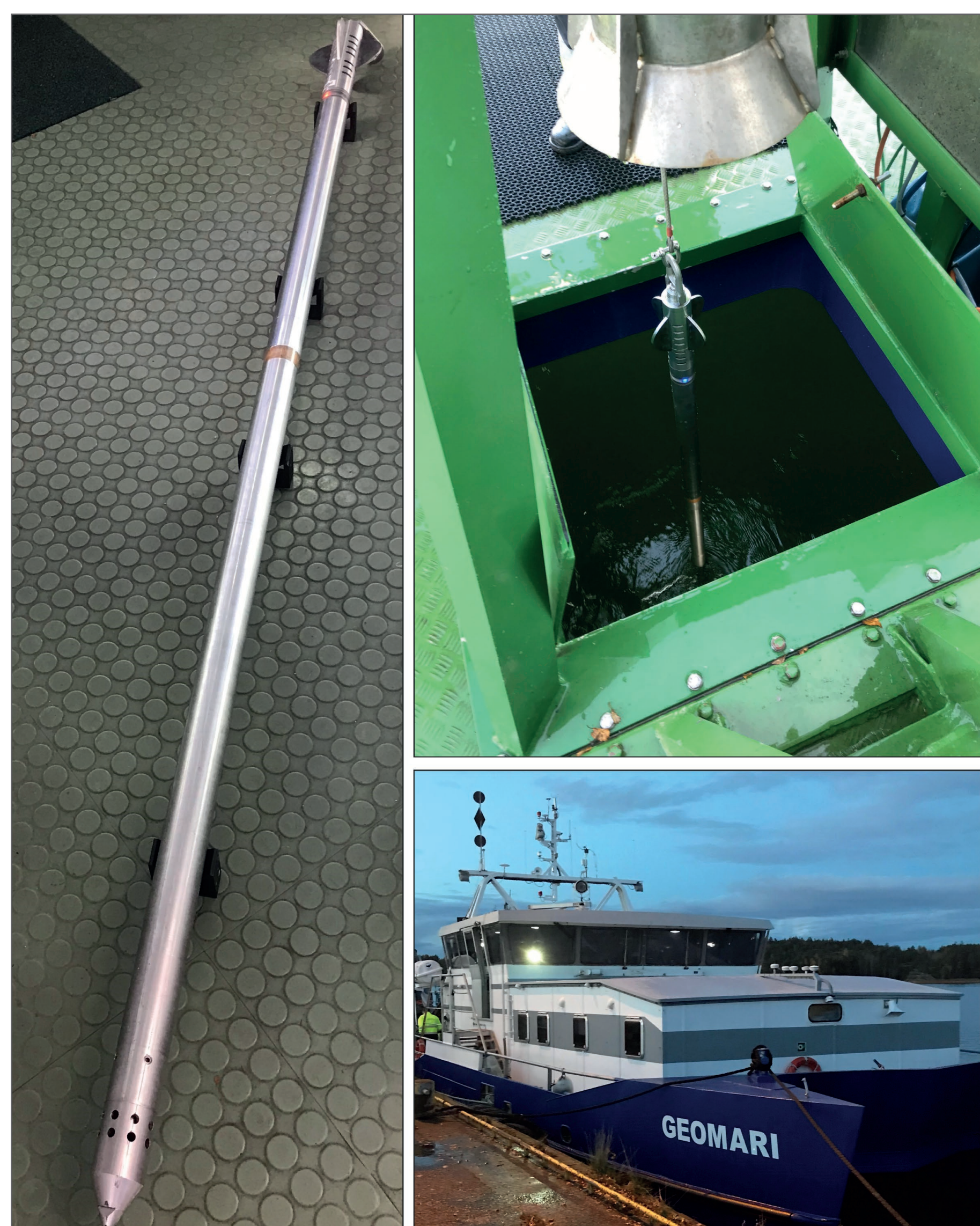
Fig. 2. Graviprobe FF-CPT instrument onboard R/V Geomari is part of the FINMARI research infrastructure.
