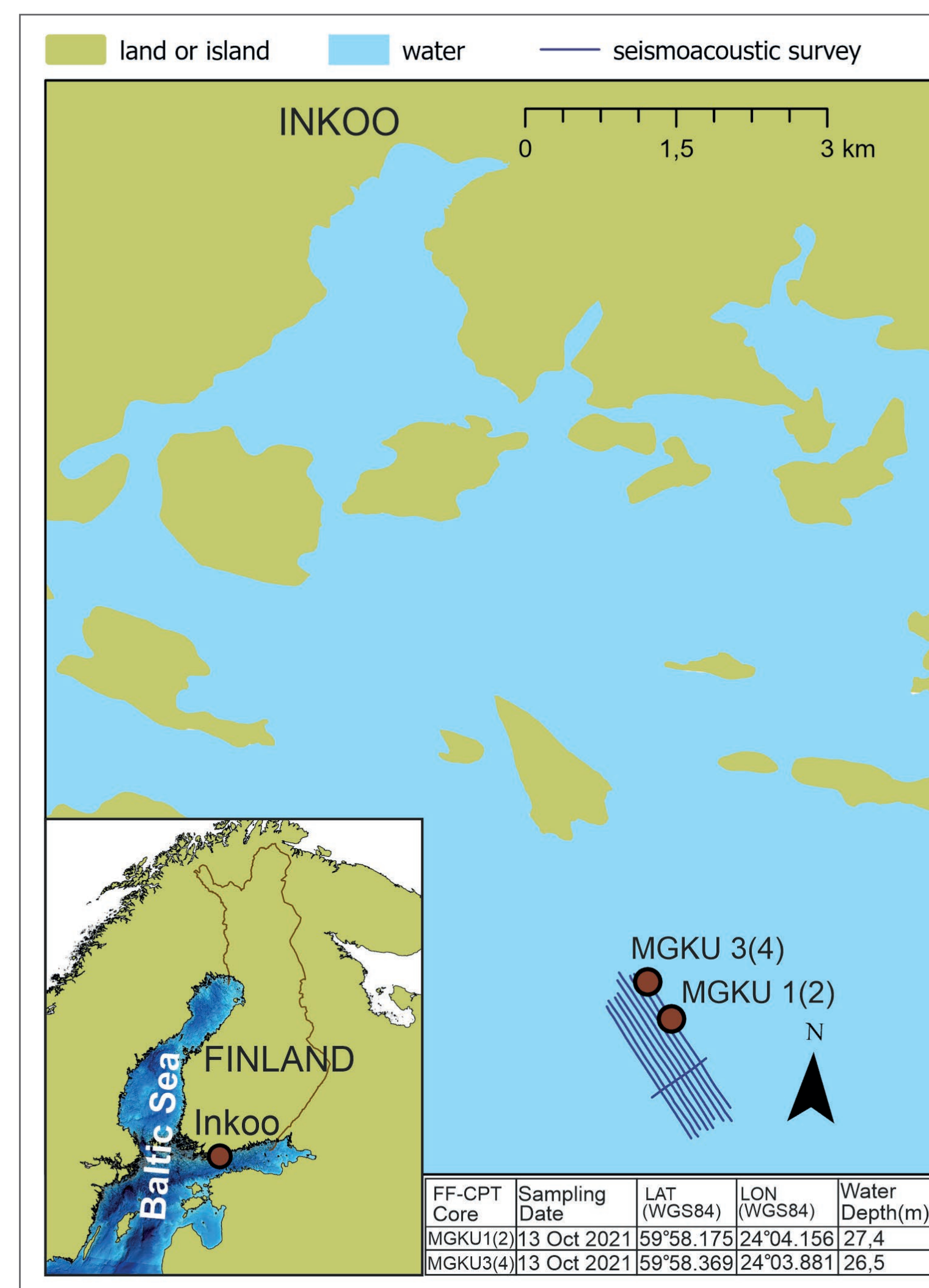
Fig. 1. Inkoo study area in the Gulf of Finland. Sediment cores were collected, and FF-CPT tests carried out at the MGKU 1(2) and MGKU 3(4) sites.
