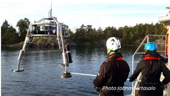
Deployment of the benthic lander in Tvärminne
