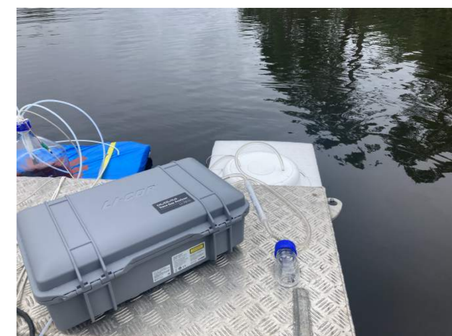
Fig. 2: Deployment of the chamber of accumulation equipped with the LI-7810.
