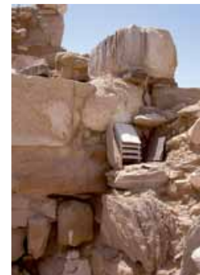
6. The open air sensor of the Hobo datalogger. Photo: Susanna Eklund 2005.
