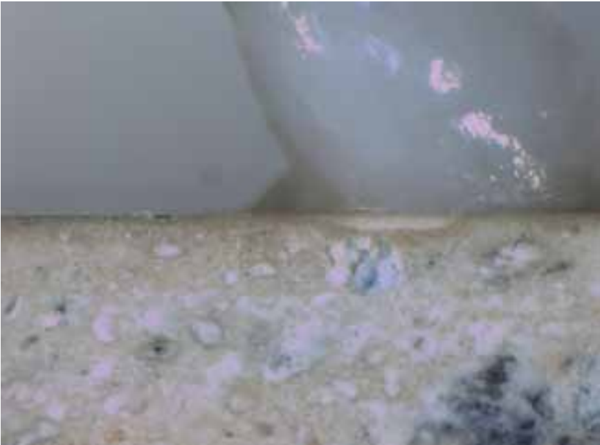
4. Cross-section of the North Hall scagliola with soap emulsion on top. Polished surface makes the top layer of gypsum glassy and turpentine or soap doesn't impregnate to the structure. (40X).
