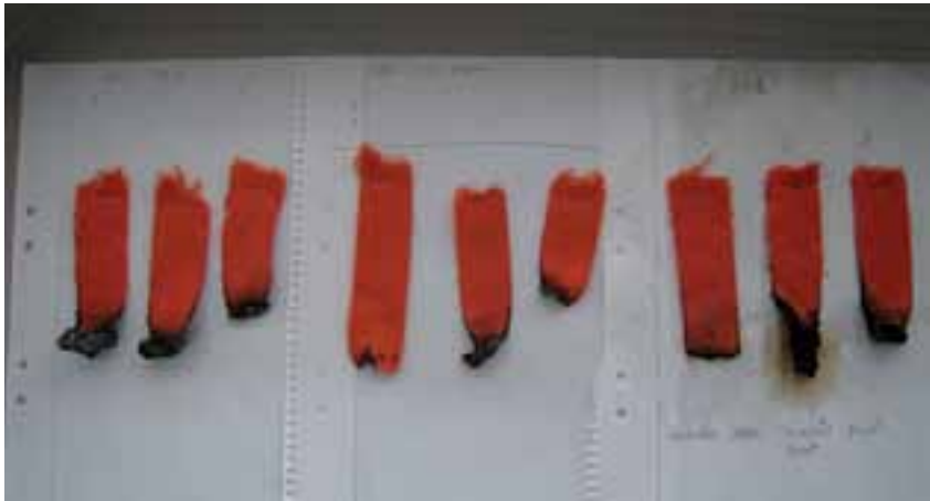
3. The untreated orange fabric (specimens in the middle) showed a better flammability resistance than samples of the same fabric treated with flame retardants Apyrum (to the right) and Secura to the left. Note the moisture spots from Apyrum. Photo: Margareta Bergstrand.
