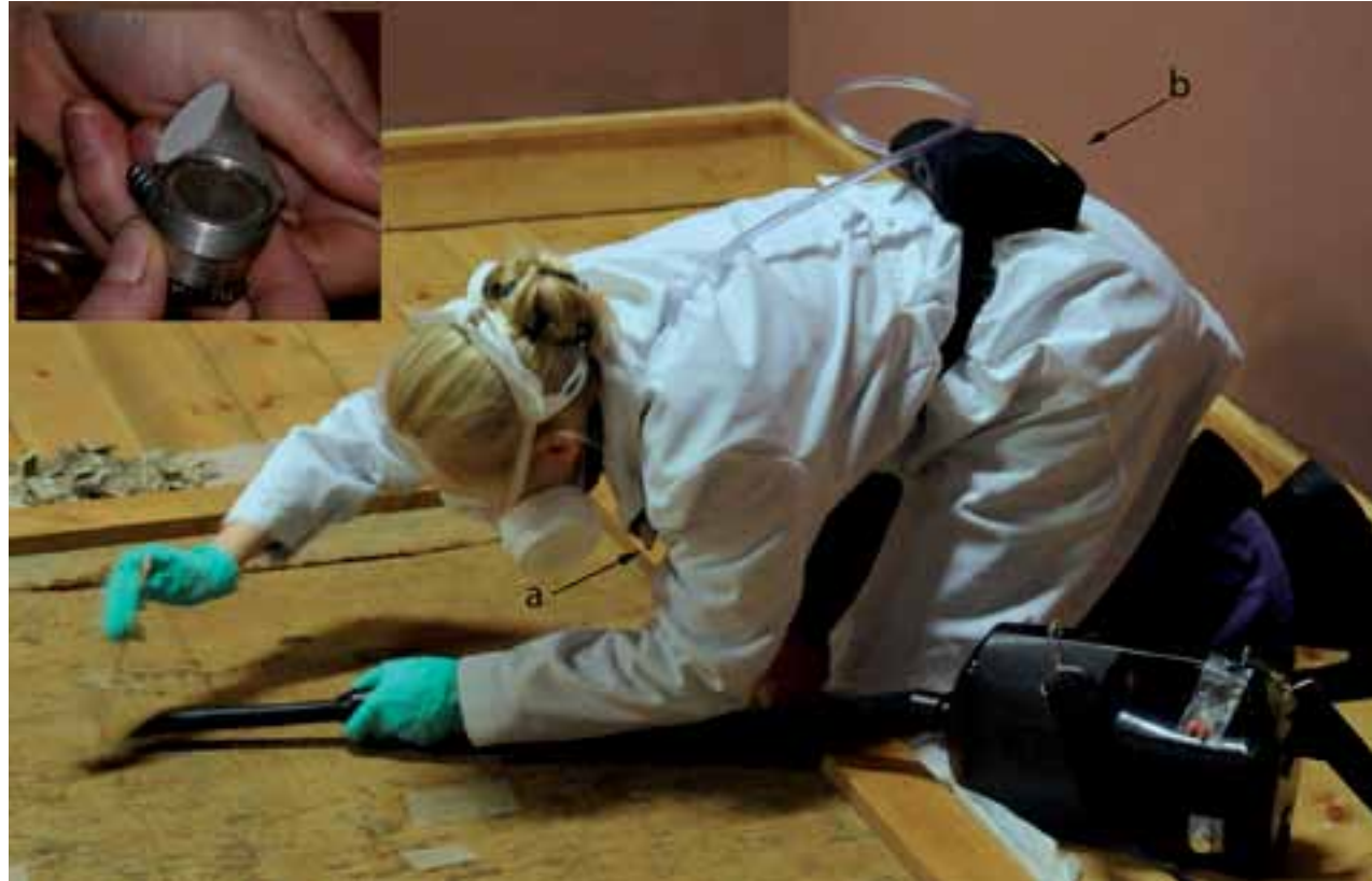
4. Magnhild with a personal air sampler. The sampler (a) is positioned as near to the breathing zone as possible, the air pump (b) is positioned at the back with a belt to allow freedom of movement. The insert shows the filter holder in the sampler.
