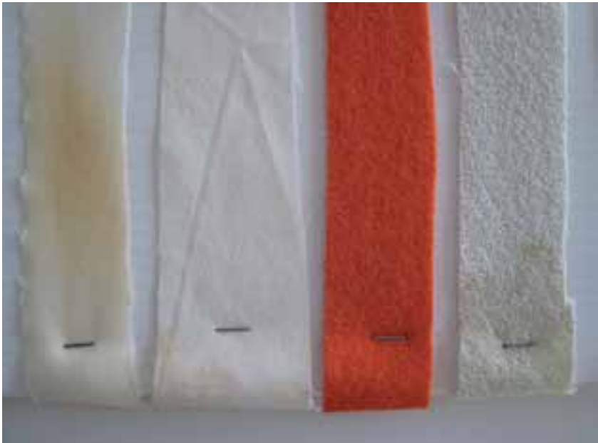
7. Samples exposed to natural light. Effects of Secura on test weave (to the left), orange and sand-coloured fabrics. Salt migration in the lower parts of the test weave and sand-coloured fabric. To the far left, brown discolouration on test weave treated with Apyrum. Photo: Margareta Bergstrand.
