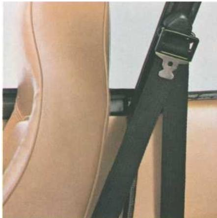
Three-point retracting seat belts are standard for the bucket seats. When the car is in use, seat belts should never be found in this position.
