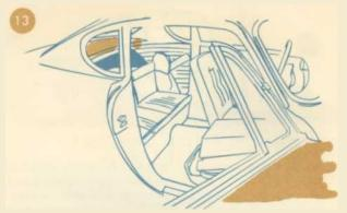
Besides the two bucket seats, interior appointments include two seats in the rear, a fully carpeted floor and a large, recessed parcel shelf behind the rear seats. Each of the bucket-seat backs folds down completely out of the way for access to the rear seats, which are large and comfortable enough for steady use by children up to high-school age and for occasional use by adults of all but the largest proportions.
