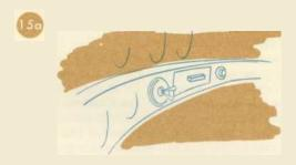
Also included in the row is a flip switch to engage overdrive. Overdrive is an optional feature that in effect provides a fifth forward speed. The four normal forward gears are used for acceleration and the overdrive is employed as a "cruising gear." The clutch does not have to be depressed when engaging overdrive since it is activated electrically merely by flipping the switch.
