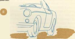
The bumpers are wrapped around the front fenders to provide more-than-adequate protection from high curbs, narrow garage doors, inconveniently placed trees and other obstructions. Additional protection to the body is afforded by a contoured chrome rub railing that terminates in a dramatic upward sweep.
