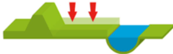
Lowering the flood plain
