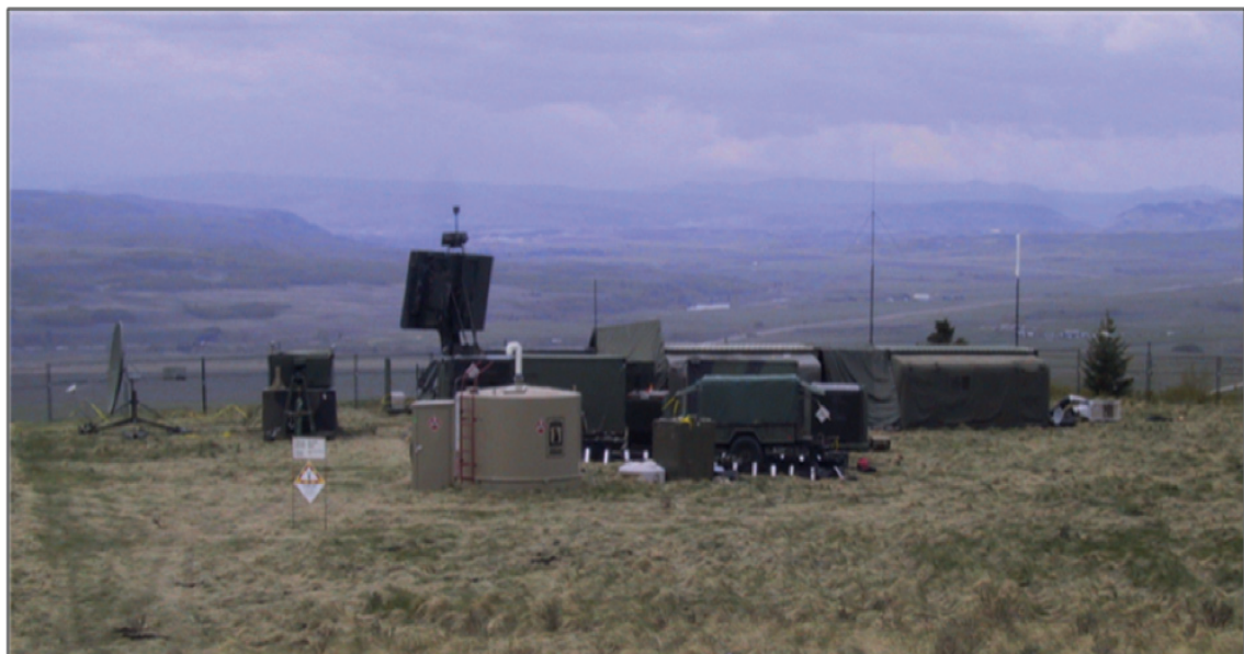
RCAF TPS-70 Mobile Radar deployed. Kuva: Canadian Armed Forces.
