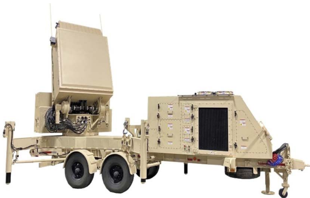
GhostEye MR™ – a new medium-range air and missile defence radar for NASAMS.
