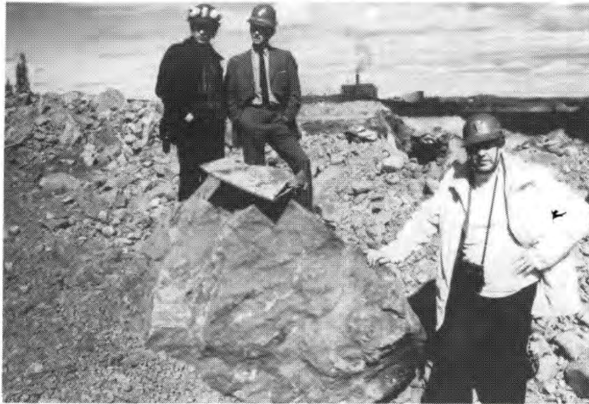
Figure 12.1. Flyrock can be thrown remarkable distances. This 3 ton boulder was thrown more than 300 m from the blast.
