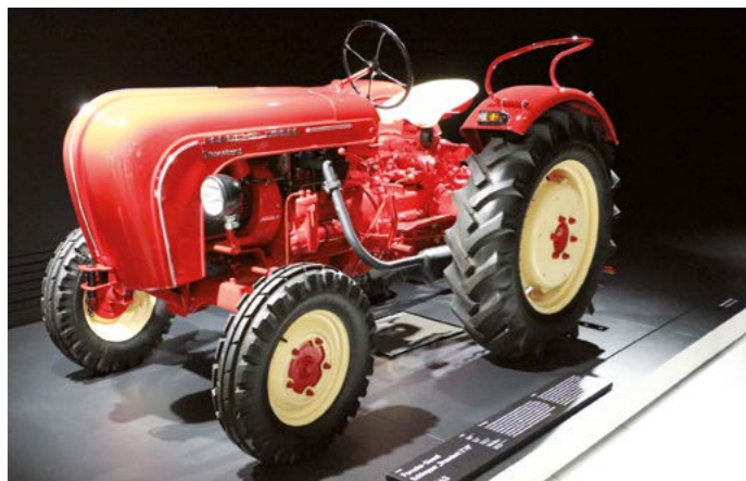
Porsche-Diesel Schlepper "Standard 218" vm. 1959, 2-syl, 1644 ccm, 18 kW (25 Hv), 20 km/h
