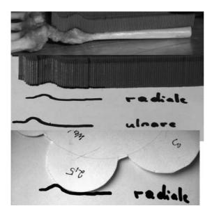
Figure 1: measuring method to quantify the profile of the volar distal radius by using a profile gauge.
