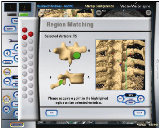
Figure 5: Region matching. Predefined regions have to be registered, so the deformable model of the vertebral bone can be fitted to the individual patient's anatomy.
