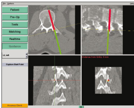
Figure 1. Example of CT-based navigational feedback This screenshot shows a CT based navigation during pedicle screw placement where the optimal location for the screw in L2 has been planned pre-operatively (red line) and the current position and orientation of the instrument used to prepare the screw canal is overlaid as a green line, facilitating precise alignment of the instrument with the plan.
