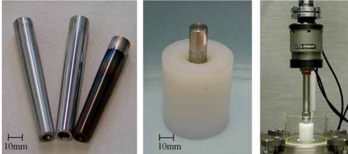
Fig. 1. (A) Cemented femoral stem-shaped metallic pins (from left to right): non-AD coated (rough), non-AD coated (smooth) and AD-coated. (B) Metallic pin specimen fixed with bone cement on a nylon block mantle. (C) A specimen mounted in the test chamber without serum lubricant.
