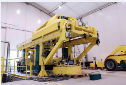
Figure 2. Bentonite buffer installation equipment, as developed by Posiva Oy within the LUCOEX project. (Photo: Posiva Oy)
