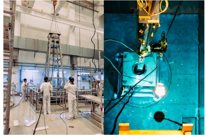
Figure 3: The combined PGET-PNAR measurement rack. Left: Lifting of the rack into the pool at the spent fuel storage. Right: Measurements ongoing in the pool. Photos: TVO
