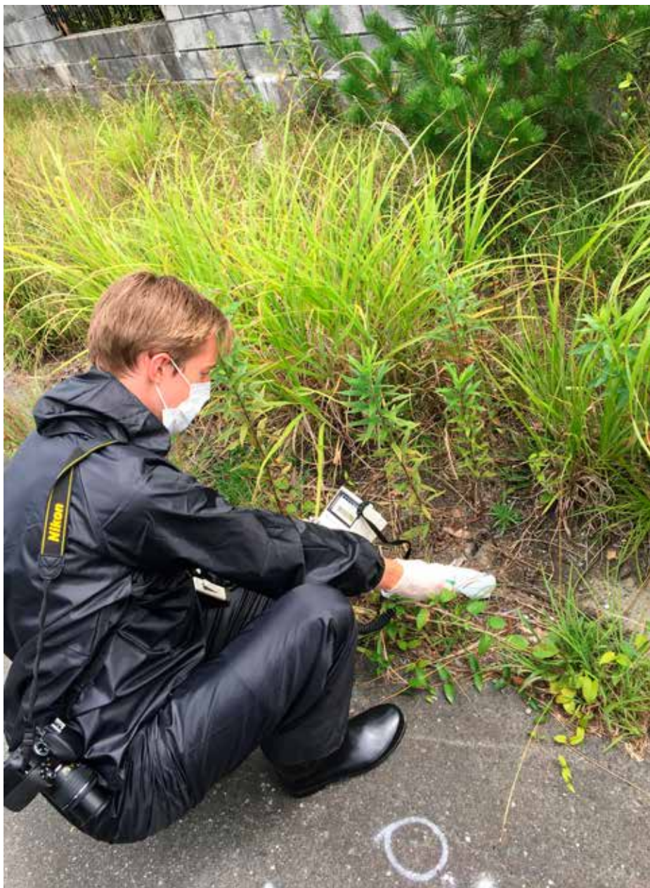
Dr Will Bower surveying roadside dust samples for Cesium-rich Microparticles in the Fukushima Daiichi Nuclear Exclusion zone.
