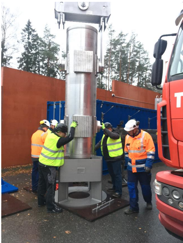
Figure 4: DNT21 cask being placed in its vertical stabilization frame for e.g. loading underwater in a pool on an NPP site.
