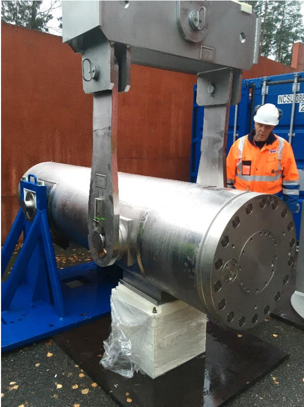
Figure 3: DNT21 handling in turning frame using lifting beam and lugs hung from a mobile crane.
