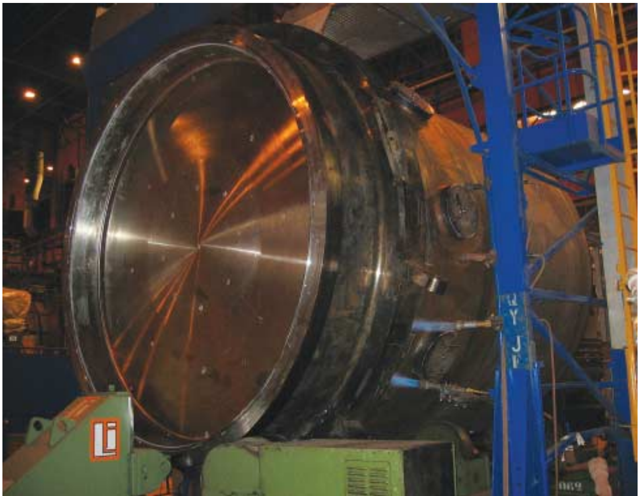
Steam Generator tubesheet is welded to the lower shell. Heat transfer tubes 5980 pcs will be welded to tube sheet in Chalon factory France.
