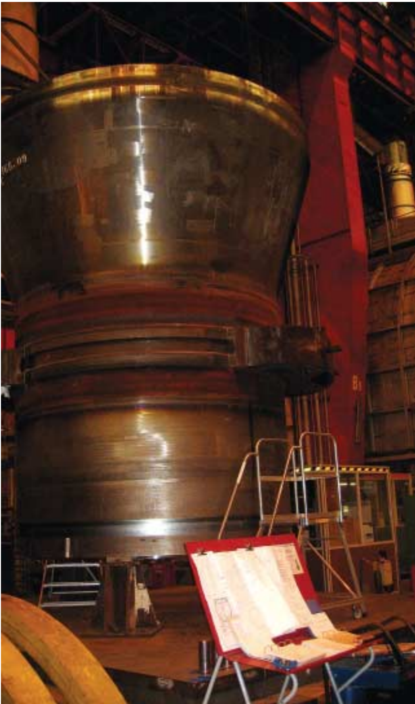
Steam generator consists of nine forgings. In the picture the first two shells are welded together in Chalon factory France.
