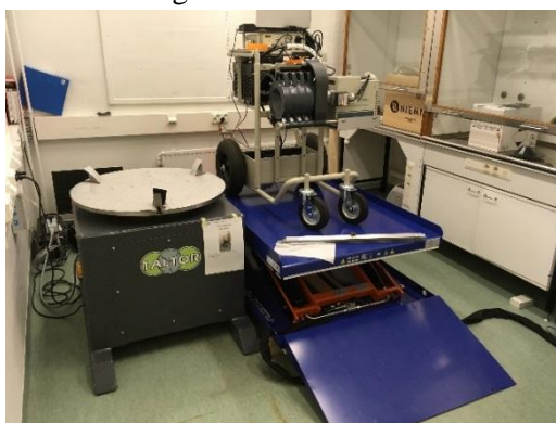
Figure 5: Rotating gamma-spectrometric measurement setup.
