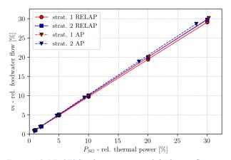
Figure 4.3 BZ OTSG relative power and feedwater flow rate trends, featuring RELAP5/Mod3.3 and Apros results.
