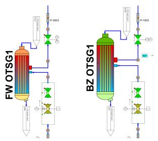
Figure 4.1 Steam generator pair of the WCLL plant in Apros.
