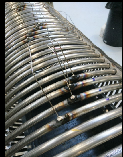
Thermocouple measurements in the MOTEL steam generator tubes
