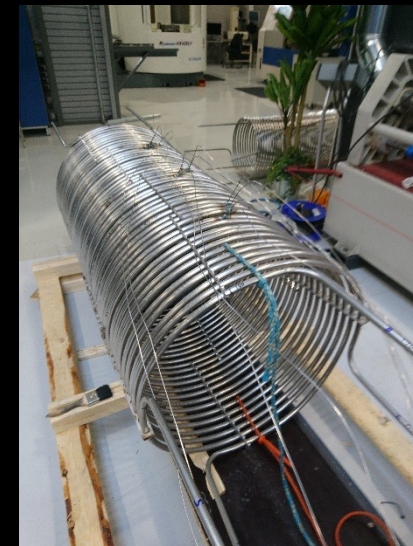
Thermocouple measurements in the MOTEL steam generator tubes
