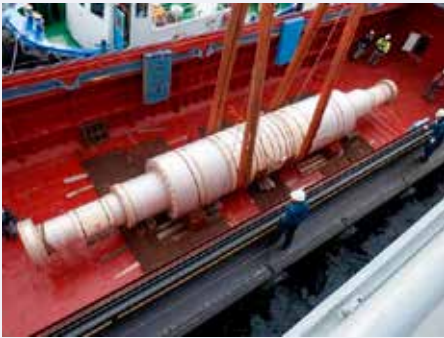
Figure 5. Generator shaft forging lifting out from a barge.
