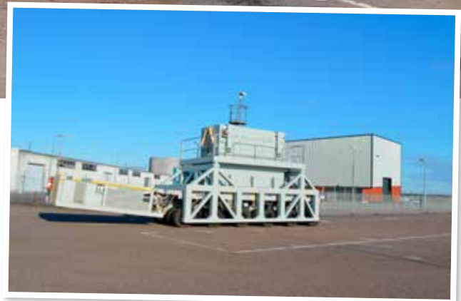
270 metric ton generator stator on its way to the barge for transport from Barsebäck to recycling company (photo: Jinert).
