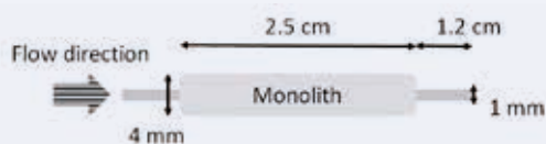
Figure 1. Principle and dimensions of the chromatographic microsystem.
