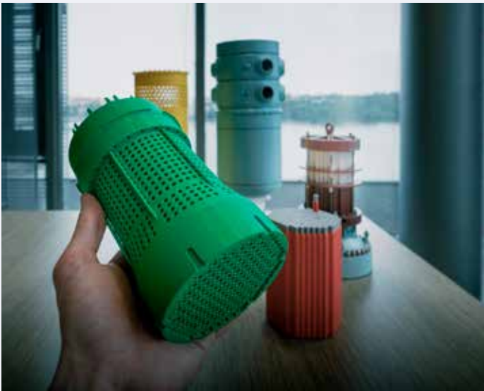
Figure 4. 60 cm tall and fully disassembled Hanhikivi reactor hands-on model printed in 1:35 scale.
