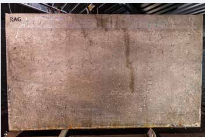
Figure 3. (a) Experiments with accelerated aging processes of mock-ups of containment structures are used to generate valuable data required for understanding ISR. (b) Crack mapping is important to understand the development of the ageing mechanism [8].
