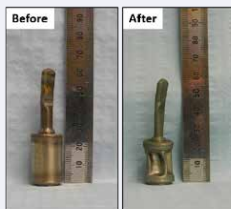
Figure 3: Pu containing HIP canister before and after processing (Taken from [5]).
