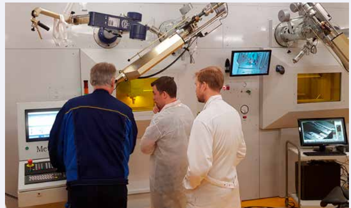
Figure 3: An important milestone was the successful fully-remote recovery of a test specimen series from the surveillance package of one of the domestic plant operators. The in-cell CNC machining station positioned inside the heavily-shielded reception hot cell, made by Finnish company Metecno Oy, was a key device in the precise operation.
