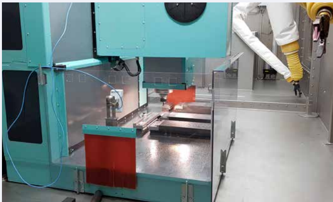
Figure 3: An important milestone was the successful fully-remote recovery of a test specimen series from the surveillance package of one of the domestic plant operators. The in-cell CNC machining station positioned inside the heavily-shielded reception hot cell, made by Finnish company Metecno Oy, was a key device in the precise operation.
