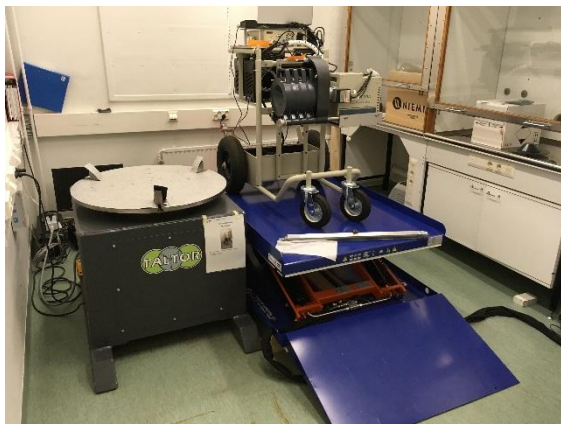
Figure 5: Rotating gamma spectrometric measurement setup.
