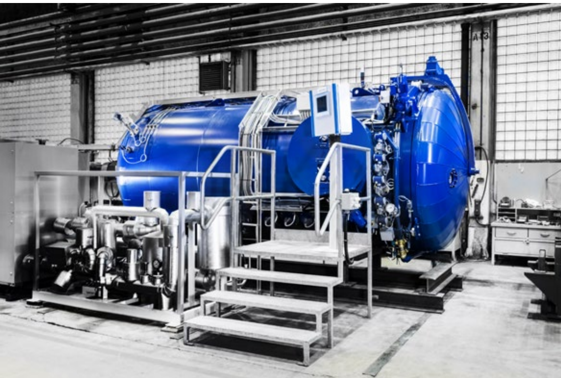
Autoclave by Platom Oy for processing uranium hexafluoride UF 6 (Platom).
