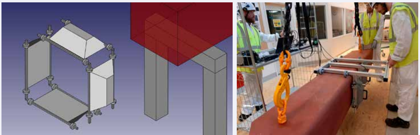
Figure 4. First design model of the measurement rack and the final rack in use (photo: Antti Rätty, VTT).
