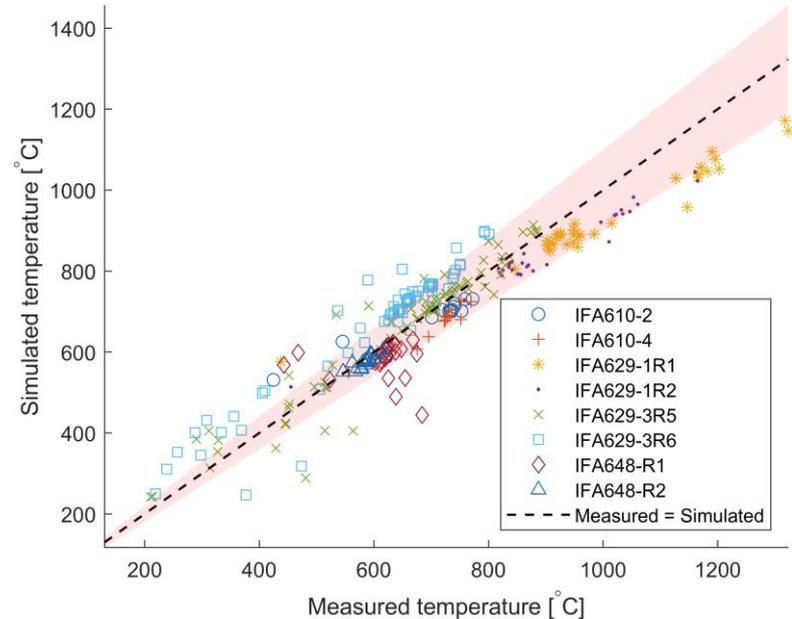
**Above:** Masterplot showing the measured vs. predicted fuel centreline temperatures with optimized  $h_{cc}$ .
