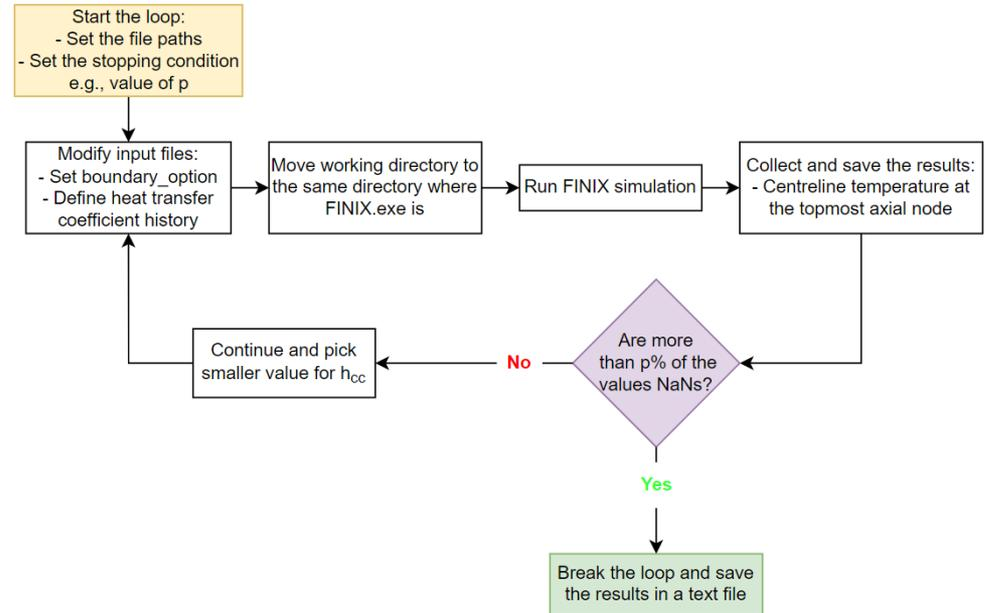
**Above:** Diagram explaining the logic of the boundary option testing script.
