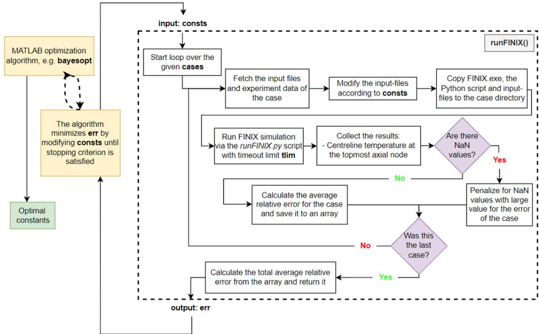
**Above:** Diagram showing the iteration logic of the optimization script.
