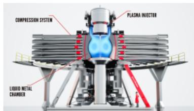
**Figure:** The Fusion Demonstration Plant (FDP) to be built by 2027 at Culham in the UK. Picture by General Fusion.
